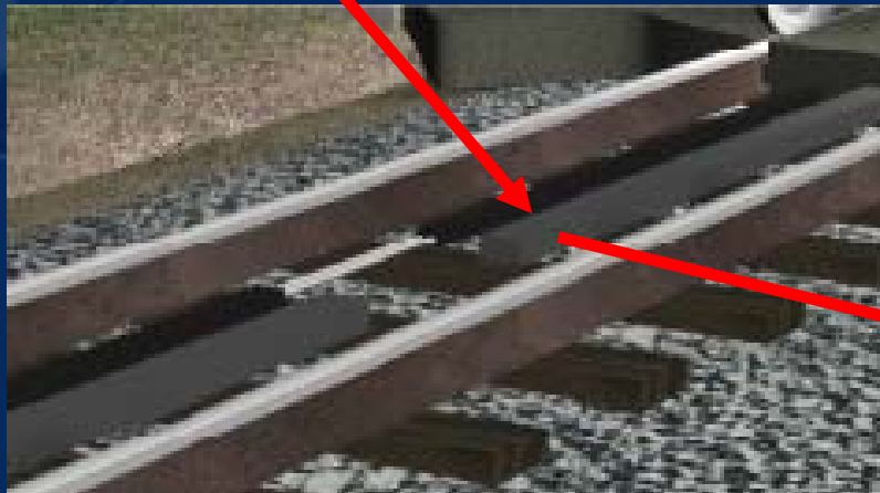
Linear motor embedded in middle of existing railway track
