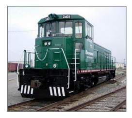
Other approaches include yard switching locomotives known as gen-sets with multiple engines that are turned on when more horse power is needed and shut down during idling.
